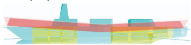
Figure 25. Compt. C,D,E or H,I,J (V1 Deep Damage)
