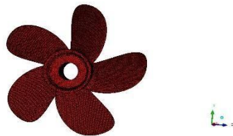
Fig. 5: Surface Grid on Propeller
