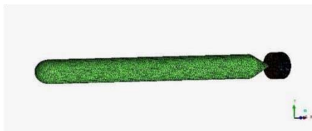
Fig. 7: Surface Grid on Hull Surface
