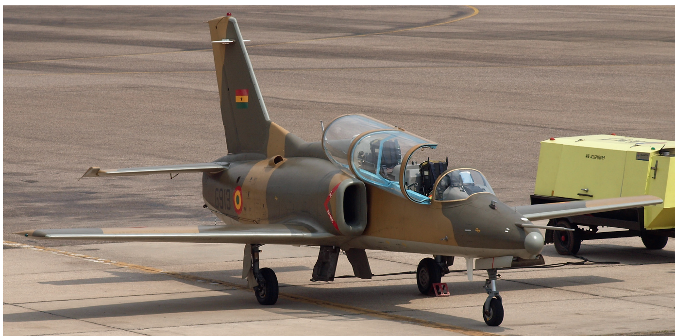
Fine study of G913, a Ghanaese K-8, the large auxiliary air inlet is readily visible on the aft fuselage. (Accra, 23 December 2011, Leonard Greer)
