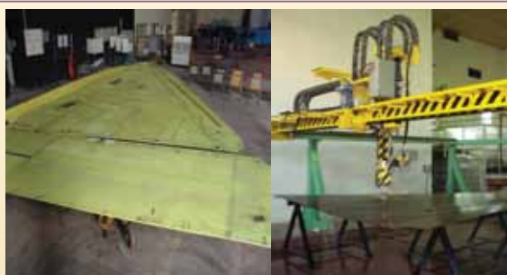
Scanning of Composite Wing Skin using Ultrasonic C-Scan System
