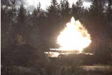
In Basic mode, employing OTA, the two interactive, dynamically compensated, vertically striking shaped charges attack the MBT from above striking down through the turret roof, avoiding the heavily protected frontal arc. The fuze system consists of both a dual-sensor proximity fuze and an impact fuze.
