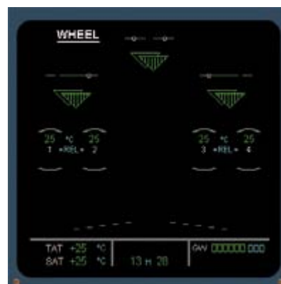
Figure 2 EIS 1 versus EIS 2 WHEEL Systems Display Page
